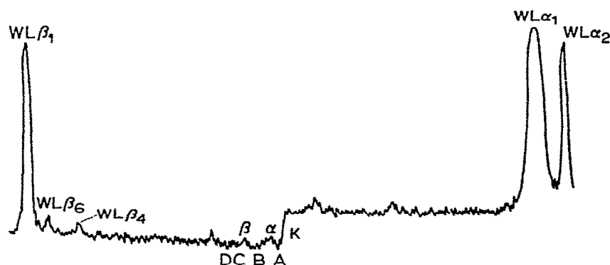
Fig. 10. Microphotometer record of K -absorption edge of copper in Cu-TPA complex.
